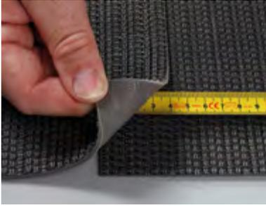
**1.** Position the strips so that the edges overlap by at least 4 cm / 1,58".
